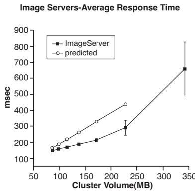
Fig. 9. Declustering effects. The process in which object were cut along their *Y – axis* and placed in different image servers results in improving the image server’s response times when the number of clusters increases
